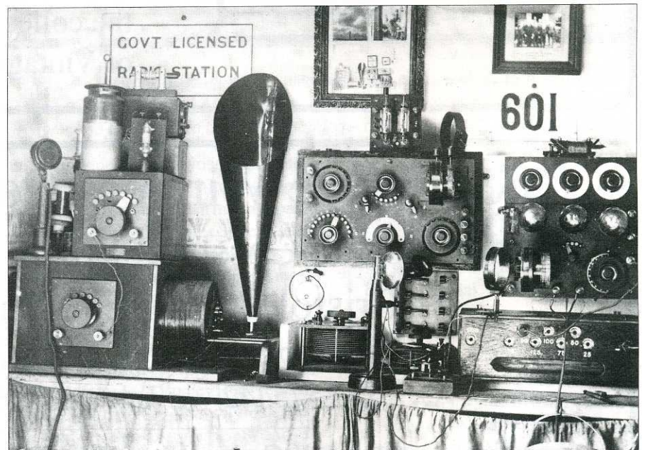
Fig. 1 - The station of Albert Pearce 6OI. Left: Transmitting equipment and home constructed loudspeaker. Centre: Receiver 1, Morse key, etc. Right: 3-valve receiver and battery box
