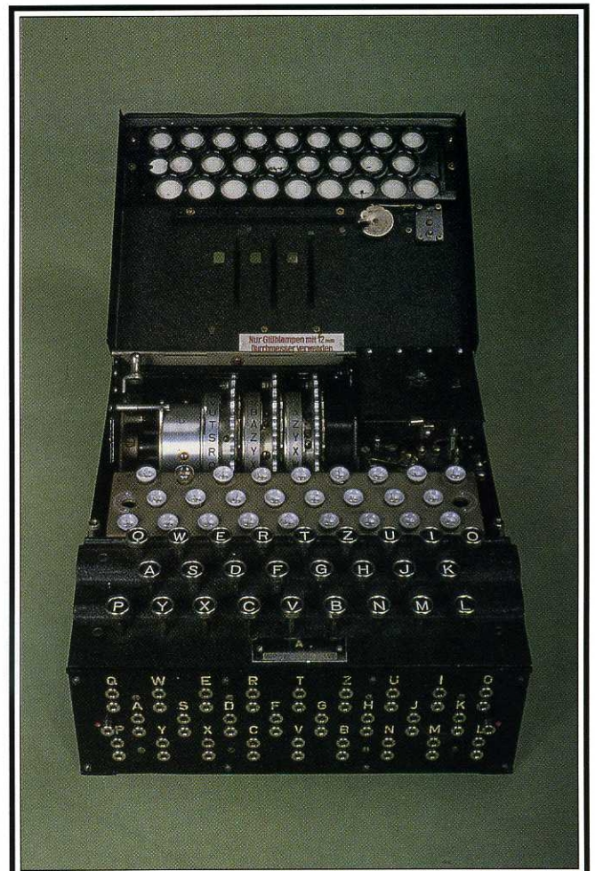
A German 'Enigma' cipher machine, with cover opened to show the rotors
