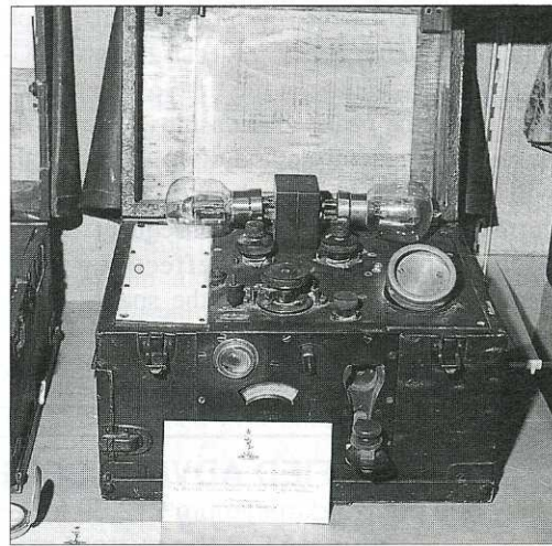
A Wireless Set Trench CW MKIII (WWI). The first all-valve transmitter, it used 'R' Type valves
