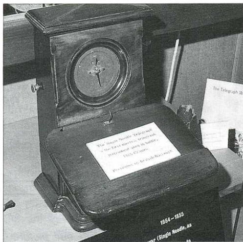
A Single Needle Telegraph (1855) as used in the Crimean War
